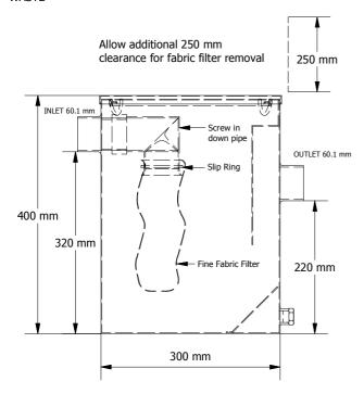
2 . Side profile - strainer basket version for food waste PARTICLES. (FILTER SOCK AND SCREW IN DOWN-PIPE REMOVED)
